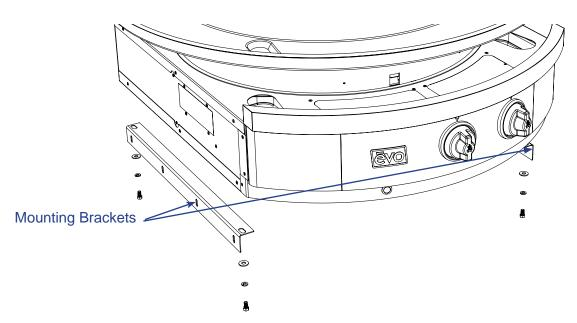
**STEP 6:** Remove two (2) mounting brackets with 7/16" Open End Box Wrench installed on Evo Affinity 30G Cooktop.
