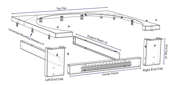
The Trim Kit for the Evo Affinity 30G is shipped partially assembled and requires installation and final assembly. Included in the kit are six (6) separate stainless steel metal components and one (1) package of hardware as listed below:
