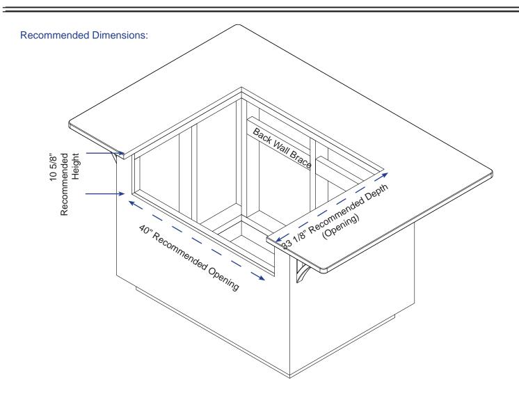
**STEP 1:** Prepare cabinet construction using either wood or steel framing. It is recommended to have a cutout measuring 33 1/8" depth by 40" width by 10 5/8" height.
